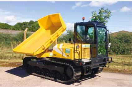
Equipped with a 180° slewing skip and rotating operators seat, allowing the operator a 3-sided tip operation and making this machine a versatile tool for material handling.
