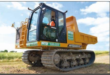
With a 360° rotation, this tracked dumper can fully tip a load at any radius. Useful on sites requiring a large volume carrying capacity where there are restrictions, such as confined routes, tunnels and riverbanks. Where turning and reversing may be a risk for the operator, this offers huge safety and environmental benefits.
