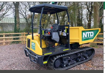
Equipped with a 180° slewing skip, the C30R-3 allows the operator to side tip from both forward tipping and rear tipping configuration. The engine complies with Tier 4i emissions/EU Stage 111B.
