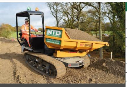
Equipped with a 160° slewing skip, the MST-300 VDR allows the operator to side tip from both forward tipping and rear tipping set up. The engine complies with EU Interim Tier 4i emissions and EU Stage 111B.
