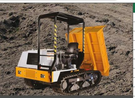
The smallest in our range. The MST-300VD is idle for small projects with restricted access. This model has drop sides, making this a good choice as a compact tool carrier.
