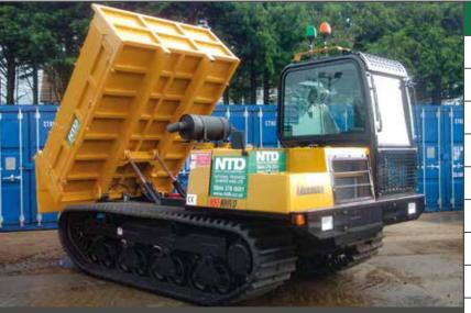
Flat body and drop down sides makes this machine a great carrier tool as well as a tip body dumper. Low ground pressure and great payload ability combined with a large fuel tank and good tracking speeds make this mid-sized tracked dumper a popular choice for many sites. Optional towing hitch available.
