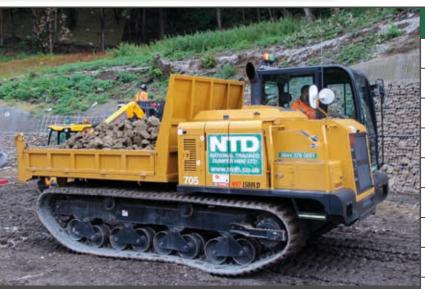
This tracked dumper offers the perfect combination of payload and performance. These rigid rear tip tracked dumpers are ideal for working in construction, environmentally sensitive, agricultural and recreational sites. They have great traction in adverse ground and can travel on steep inclines where a wheeled dumper struggles. Offering low ground pressure rubber tracks, ensuring reduced soil compaction.
