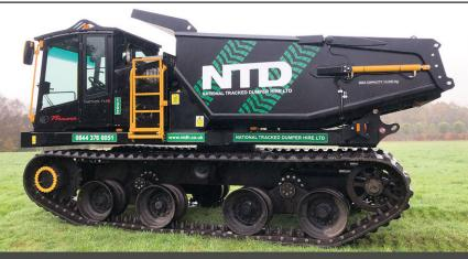
This impressive sized tracked dumper offers the highest speed combined with the highest payload in its class and will set new standards for productivity and mobility. With its 13,200 kg capacity, this rubber tracked crawler carrier has the largest payload of any vehicle of this type in its category.
